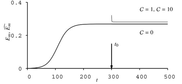
**Figure 1.** Evolution of magnetic energy  $E_m$  for  $t < t_0$  governed by the system (1) and (5) for  $\mathcal{D} = -10$ . In the moment  $t_0 = 300$  the new magnetic field  $(\hat{A}, \hat{B})$  with the initial conditions defined by constant  $C$  is switched on, see (6) and (5). Plots for  $E_m$  and  $\hat{E}_m$  (with  $C = 0$ ) for  $t > t_0$  coincide. All the solutions are stationary.
