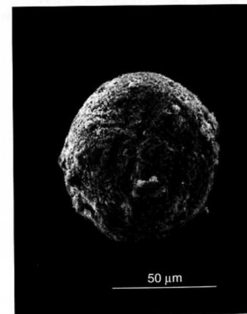
Figure 10.6 Electron micrograph of an iron-rich magnetic spherule collected from the topsoil 800 m from Jaworzno power station (Poland). (Courtesy of Tadeusz Magiera.)
